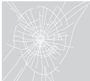
< Broken Laminated Glass >
